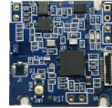
DC-DC/Battery Charger/BLE (DA14680)
